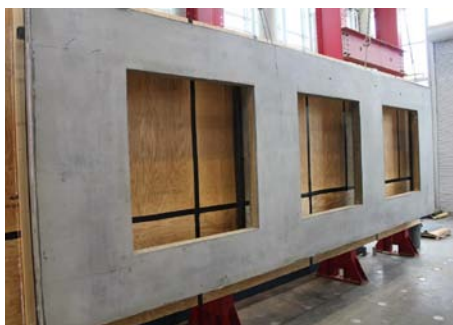
CarbonCast Insulated Architectural Cladding panel under-going load testing at North Carolina State University
